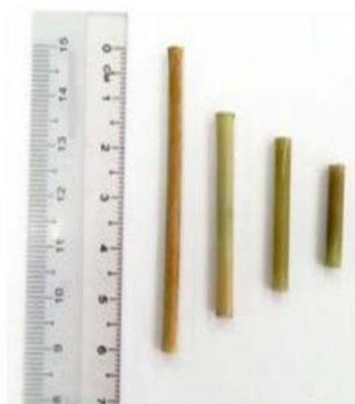
Fig. 1. Samples of bamboo with different lengths of stem.
