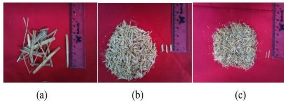
Fig. 1. Betung bamboo particles of various sizes: a) wool, b) medium, and c) fine
