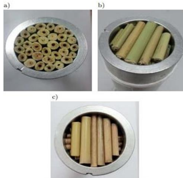
Fig. 3. Arrangement of bamboo in impedance tube: a) axial arrangement, b) transverse arrangement, and c) cross transverse arrangement.
