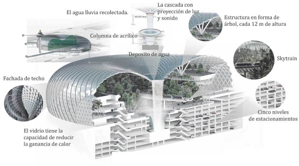
Figura 4. Corte Transversal Edificio La Joya Adaptado de: News Channel Asia (s.f.). Inside Jewel Changi Airport, Recuperado de https://infographics.channelnewsasia.com/jewel-changi-airport/index.html .
