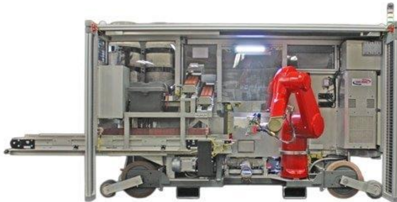
Figura 4: Sam el robot albañil. 2019. Mecanismo interno del robot. Tomado de “Construction Robotics” por Construction Robotics Advancing Construction, 2007, recuperado de https://www.construction-robotics.com/sam100/
